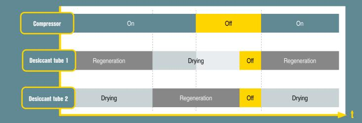
Upon receipt of a 'Remote Off' signal, the currently running regeneration phase is fully completed. Only then does the half-cycle end. This requires dried compressed air. The next half-cycle starts when the 'Remote On' signal returns. Benefit: Upon receiving a 'Remote On' signal, a lower pressure dew point will be available immediately.
