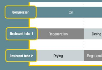
Upon receipt of a 'Remote Off' signal, the cycle will be stopped immediately. Upon receipt of a 'Remote On' signal, the cycle will be restarted.
